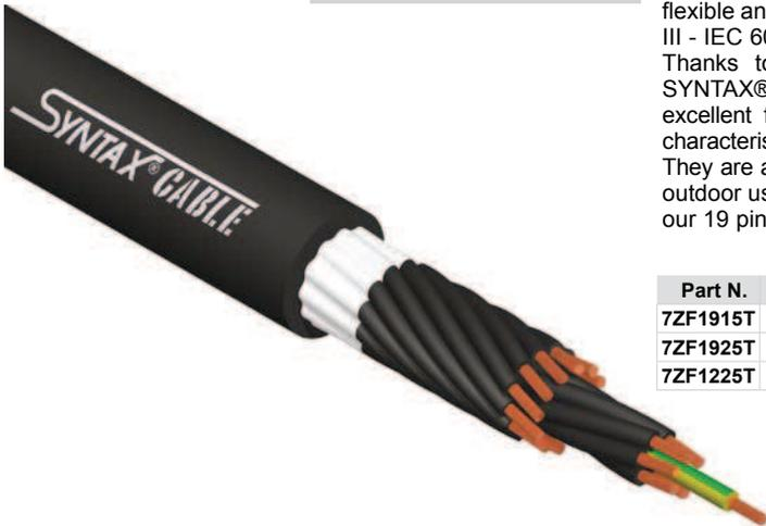
These SYNTAX® MULTICORE POWER cables are manufactured with a flexible and impact absorbing external jacket, compliant with CEE 20-22/III - IEC 60332-3-24 - EN 50266-2-4 fire resistant regulations.
